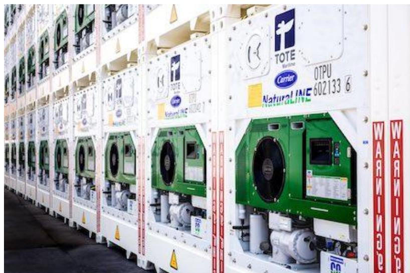
*TOTE Maritime Puerto Rico's latest investment in green technologies is the addition of 220 containers leased from SeaCube Containers and refrigerated by Carrier Transicold NaturaLINE units, which use the natural refrigerant carbon dioxide, with an ultra-low global warming potential.*
